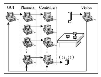
Fig. 3 Network architecture of MARS test-platform
