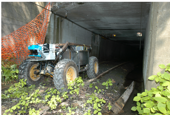
Figure 1.2: The Groundhog UGV from Carnegie Mellon University is designed for mapping underground mining tunnels.
