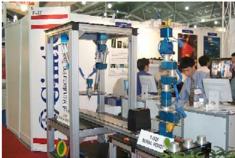
Figure 1.8: Reconfigurable robotic workcell (Nanyang Technological University)[21]
