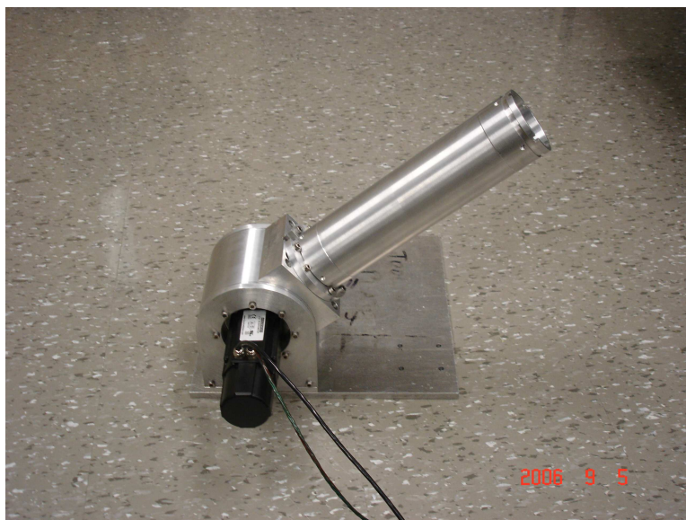
Figure 2.5: MRR rotary joint built at UW
