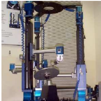
Figure 1.2: Parallel robot for machining [8]
