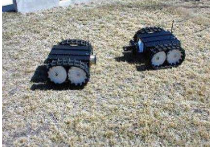
Figure 1.6: Mobile type self-reconfigurable robot [14]
