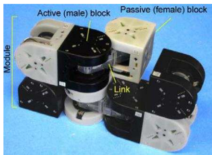
Figure 1.4: Module cell for snake-shape self-reconfigurable robots [12]
