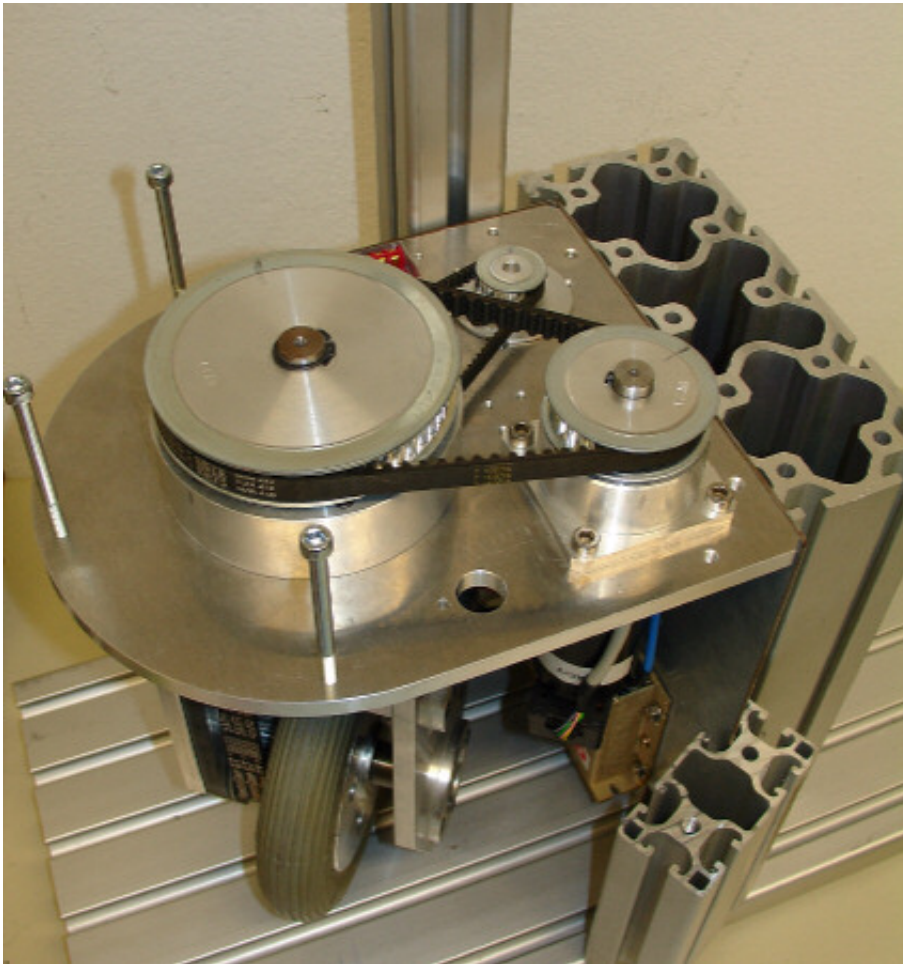
Figure 5.4: test stand with drive unit.
