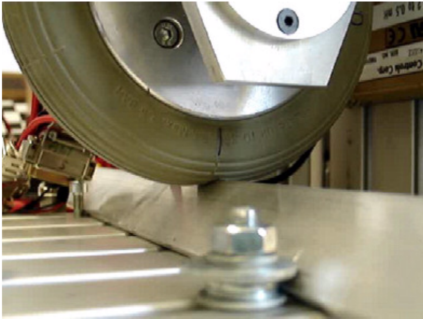
Figure 5.6: Aluminium angle piece fixed in test stand to simulate a step edge.
