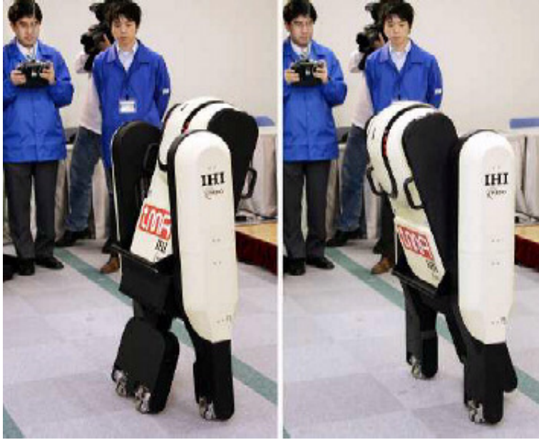
Figure 1.27: The IMR-Type 1 wheeled robot is capable of static and dynamic balance [67].
