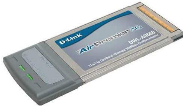
Figure 2.3: D-Link DWL-AG660 802.11a/11g 108*Mbps* Wireless PCMCIA Adapter.
