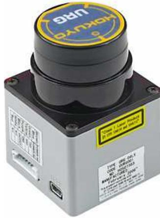
Figure 3.4: Hokuyo URG-04LX laser rangefinder.
