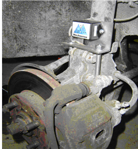
Figure 3: The accelerometer mounted on the bottom of the Toyota Tercel left front damper to measure the acceleration of the wheel-hub.
