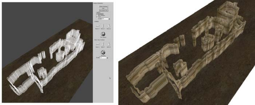
Fig. 3. The cistern located at Wignacourt Museum College Garden. This was a fairly large and complex cistern, including several pillars and stairs down into the cistern. On the left is shown the visualization system’s GUI and a wire frame of the mesh extracted from the occupancy grid. On the right is a texture mapped model.
