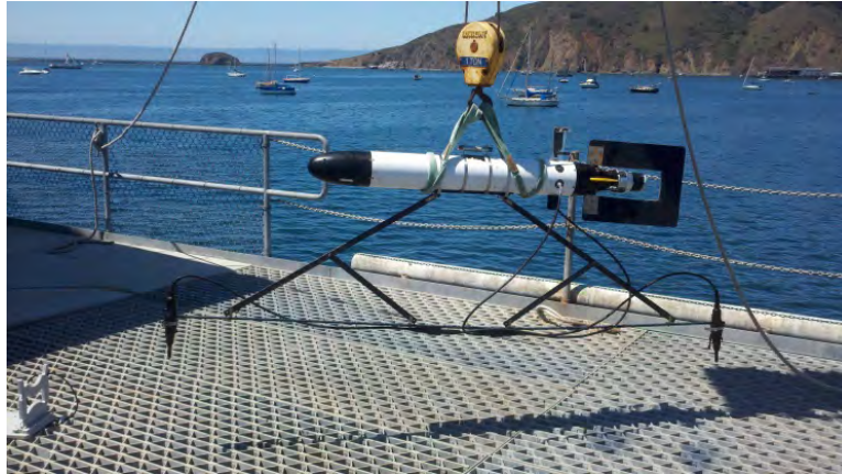
Figure 2.14: The Rig Used to Fix the Hydrophones under the AUV
