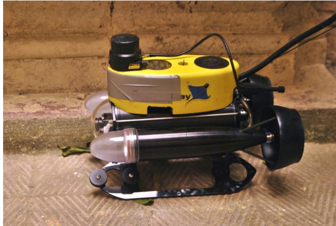
Figure 1.1: The VideoRay Pro 3 GTO is an underwater micro-ROV with dimensions 36.8cm x 28.9cm x 21.6cm. It is equipped with depth and compass sensors along with a front and a rear video camera. A Tritech Micron scanning sonar was attached to the top of the ROV.
