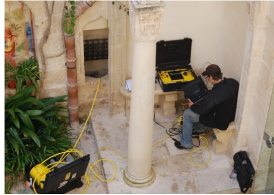
(b) Deployment of the Robot in Mdina, Malta. The robot is down in the cistern at the top of the image (where the yellow tether is emanating from), while the human operator uses the control box. The image also highlights how narrow the cistern shafts are.
