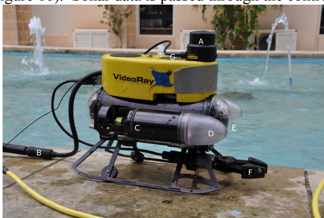
Figure 15: The Video Ray Pro III, a small ROV used for this project. Labeled parts: (A) sonar head, (B) tether, (C) forward thruster, (D) headlight, (E) video camera, (F) gripper for sample collection, (G) vertical thruster
