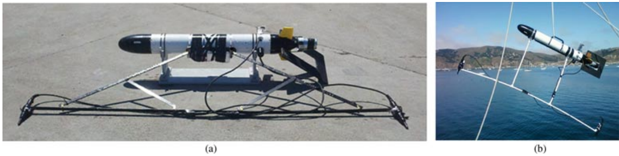
Figure 1. The OceanServer Iver2 AUV equipped with a test stereo-hydrophone acoustic receiver system. Two prototype configurations are shown. In (a), a carbon fiber frame is used to attach the hydrophones. In (b), a pvc tube frame is used.
