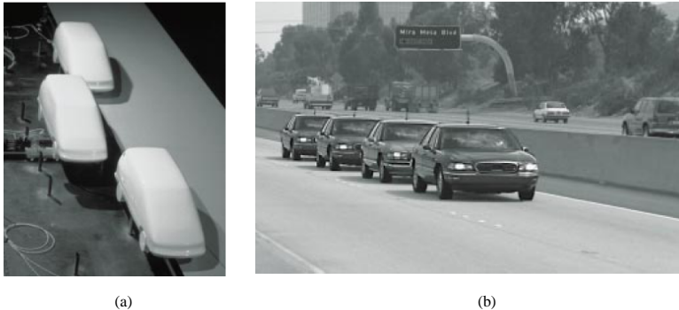
Figure 1 (a) Three-Lumina platoon in the Dryden wind tunnel at USC, and (b) platoon operation at 4-meter spacing to measure aerodynamic drag and fuel consumption (source: Browand and Michaelian, 2000).
