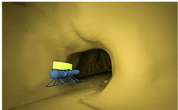
Figure 1: An ROV navigating through an ancient tunnel system in Malta (top) and corresponding render in the generated map (bottom)
